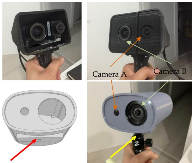
Figure 2. Initial prototype configuration P-1 (top) and the actual prototype P-2 (bottom), 14 cm long and lighter, with an extendable pole anchor point (red arrow) and a ball joint system (yellow arrow) to facilitate data capture.
