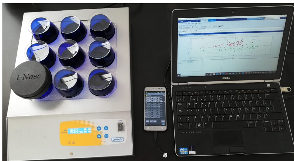
Figure 1. E-nose device and technology needed to measure samples of Californian-style black olive in a standard glass and heating block.
