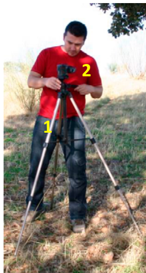
Figure 45. 1) Tripod the camera platform rests on, at a height of 1.5 m above the ground. 2) The digital camera and fisheye lens are fitted to the tripod
