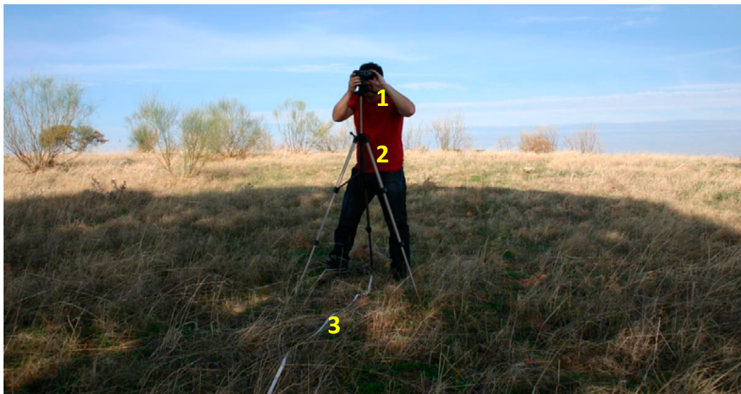
Figure 50. 1) Digital camera fixed on tripod. 2) Tripod on which the camera platform rests on at a height of 1.70 m above the ground. 3) Tape measure to measure the 10 m to the tree
