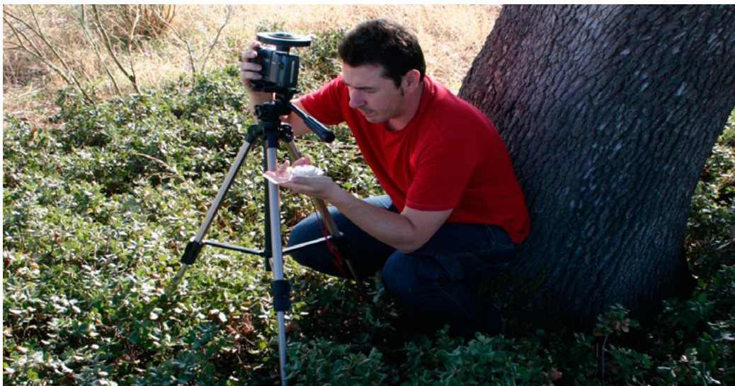
Figure 47. Positioning the photographic equipment 40 cm from the trunk, and consulting the compass to point to geographic north.
