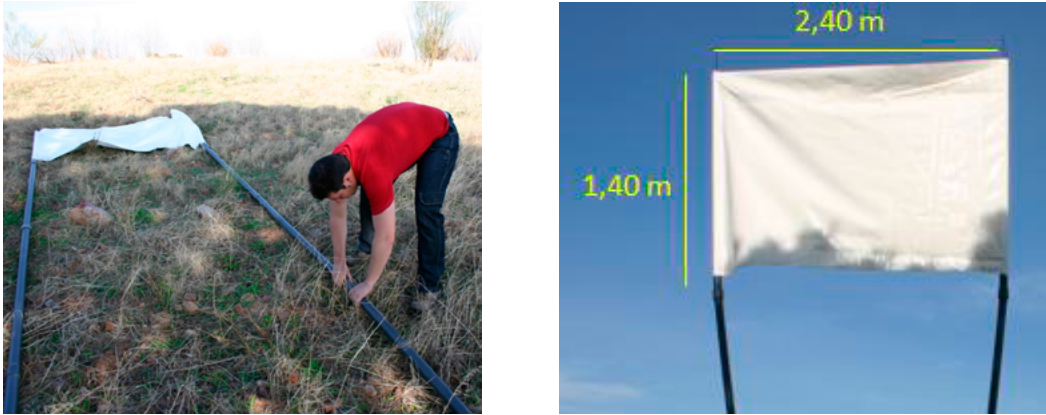
Figure 51. Left: fitting the screen to 1.5 m lengths of PVC tubing. Right: the unfurled screen which is 2.4 m wide by 1.4 m high.
