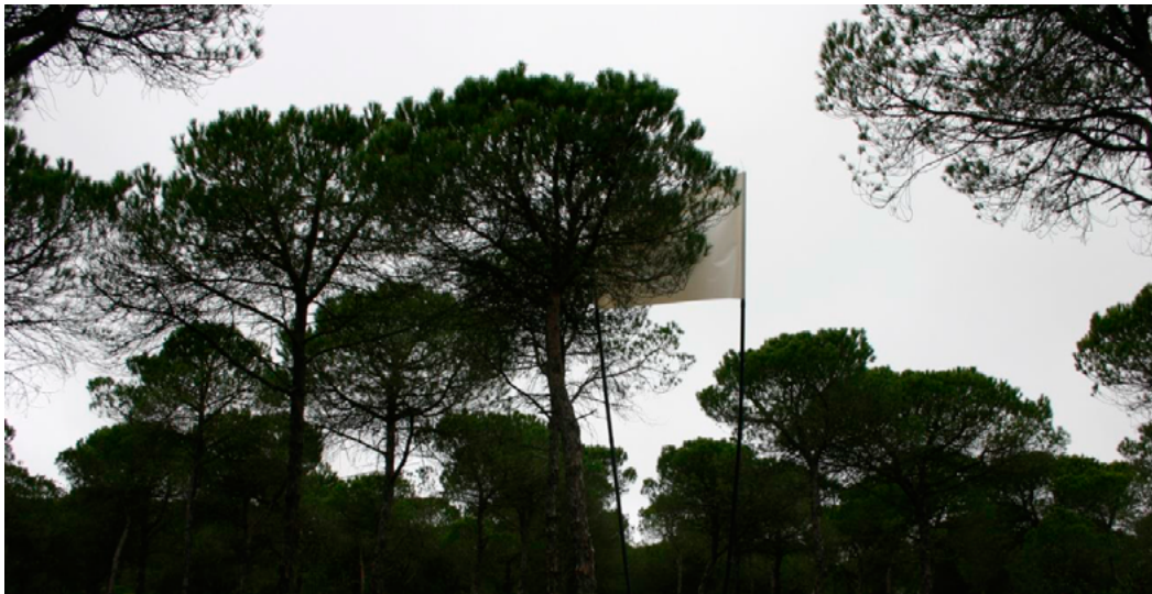
Figure 52. The screen is placed behind the tree canopy and the photos are taken from the different orientations at 10 m from the tree trunk.
