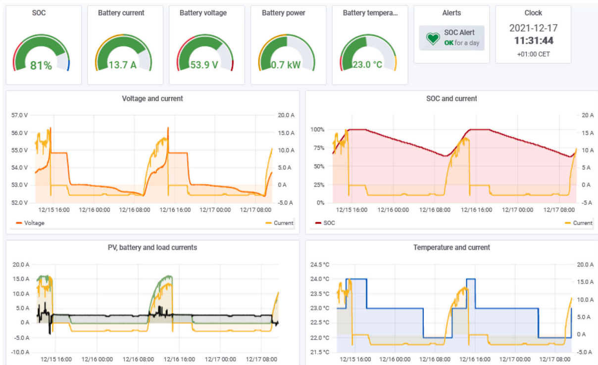
Fig. 7. Aspect of the Grafana dashboard devoted to monitoring the LiB.
