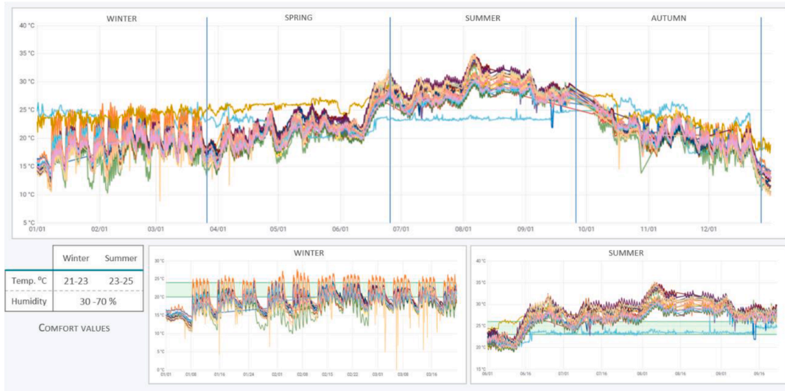
Fig. 10. Grafana dashboard with visualization adapted to the building manager with the evolution of some rooms’ temperature of one of the pavilions in 2018 with annual graphs and from winter and summer period (including comfort limits according to (Technical committee AEN/CTN 100, 2007)).
