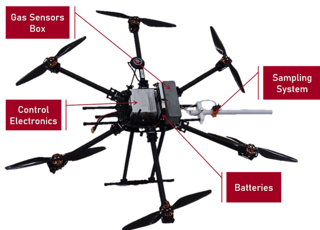
Fig. 2. Hexacopter and detail of the electronic system.
