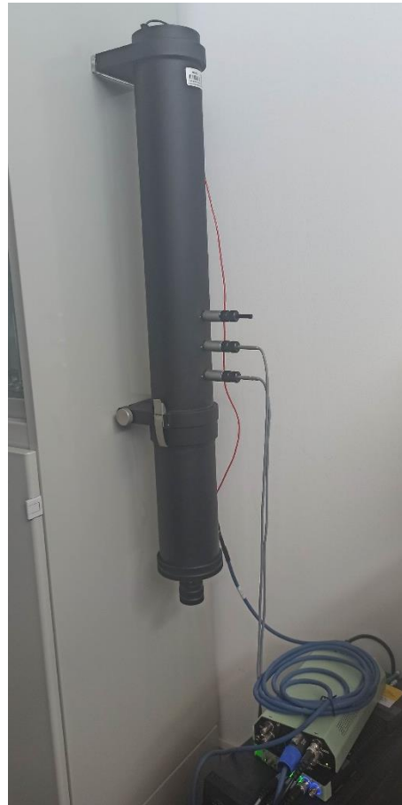
Figure 3. Impedance tube disposition used for the measurements: 100 mm holder.
