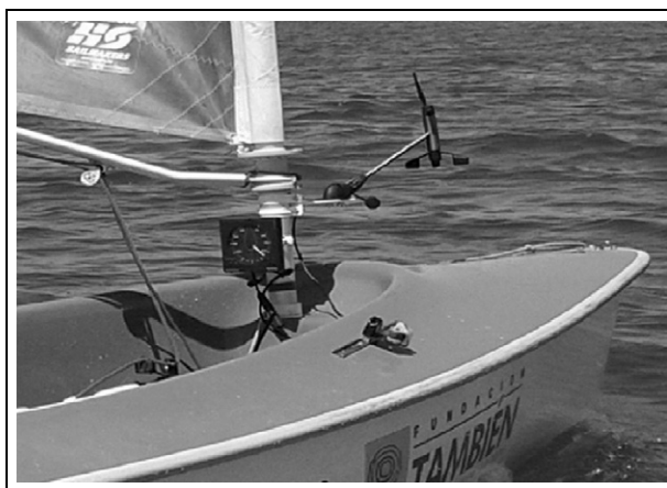
Figure 2. Wind equipment, consisting of a display panel and a wind vane, installed on the mast of the boat.
