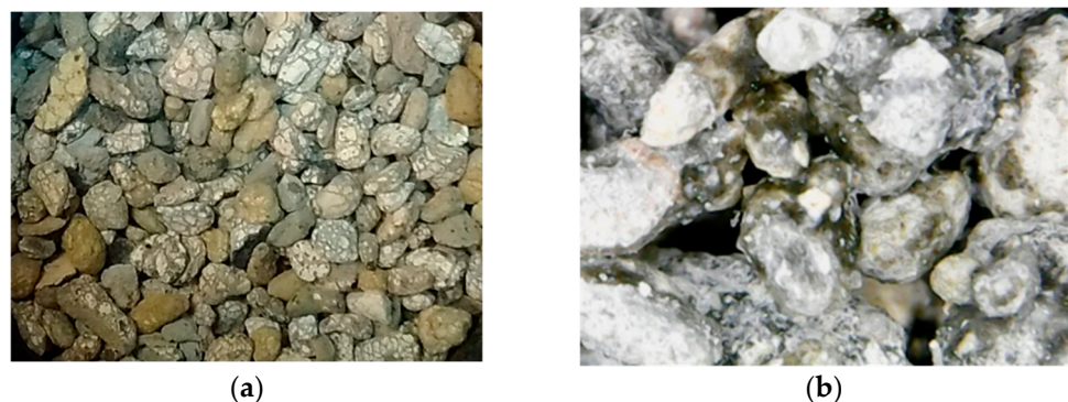
Figure 1. Expanded clay used: (a) an overall picture and (b) a more detailed image.
