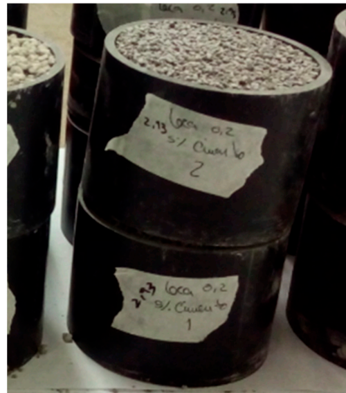
Figure 3. Porous concrete test specimens with expanded clay, prepared for impedance tube measurements.
