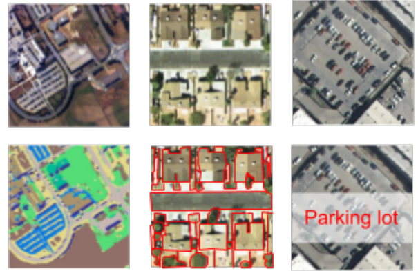
Fig. 1. Remote sensing classification can be tackled at three different levels: pixel-level (left), object-level (center), and scene-level (right)
