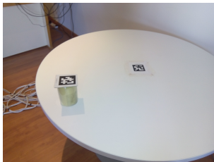
(c) Table and mug . The April-Tag marks identify and locate the objects.
