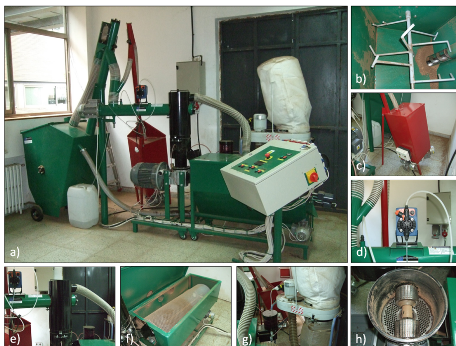
Figure 2. (a) Pelletizing equipment; (b) product hopper; (c) hopper and endless screw for auxiliary products; (d) water addition system; (e) flat die group; (f) cooling container; (g) lubrication and vacuum cleaner systems; and (h) flat die and rollers.
