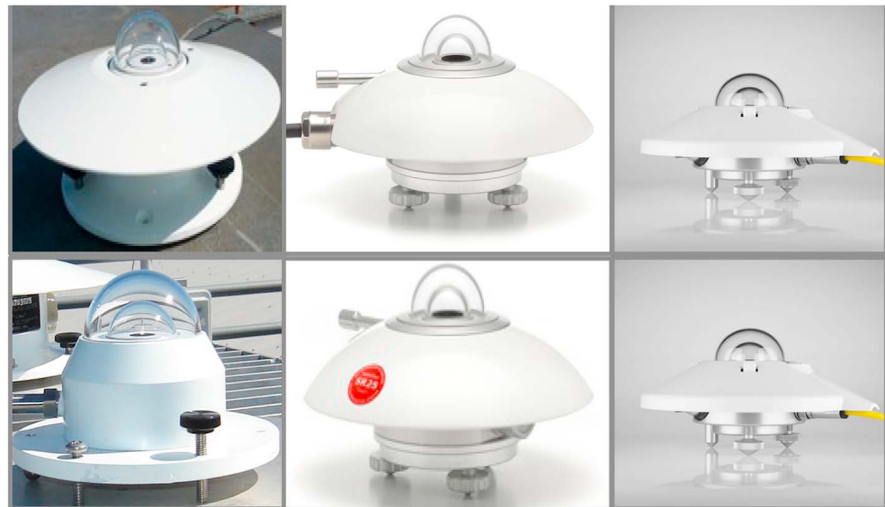
Figure 1. Participating pyranometers. From left to right:(top) SPP, SR20, and CMP11 and (bottom) GPP, SR25 and CMP22 (bottom).
