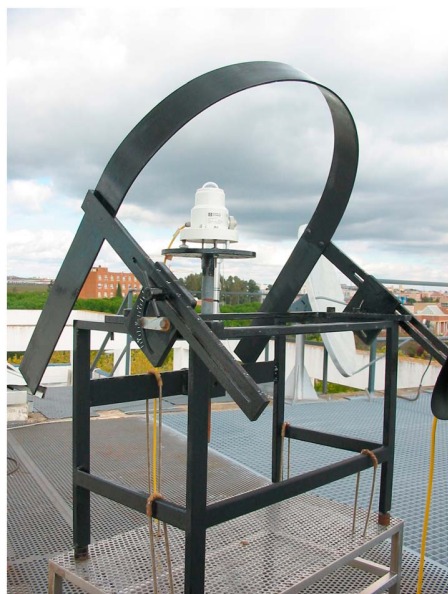
Figure 1. Shadow-band adapted for the UVS-E-T pyranometer.
