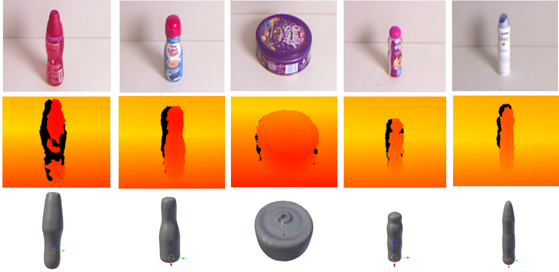
Fig. 5: Reconstruction of rotationally symmetric household objects. The top row shows a photo of the object. The middle row shows the corresponding depth image recorded using a Microsoft Kinect. The bottom row shows the completed mesh. Reconstruction was performed from a single image through the analysis of extrusions.
