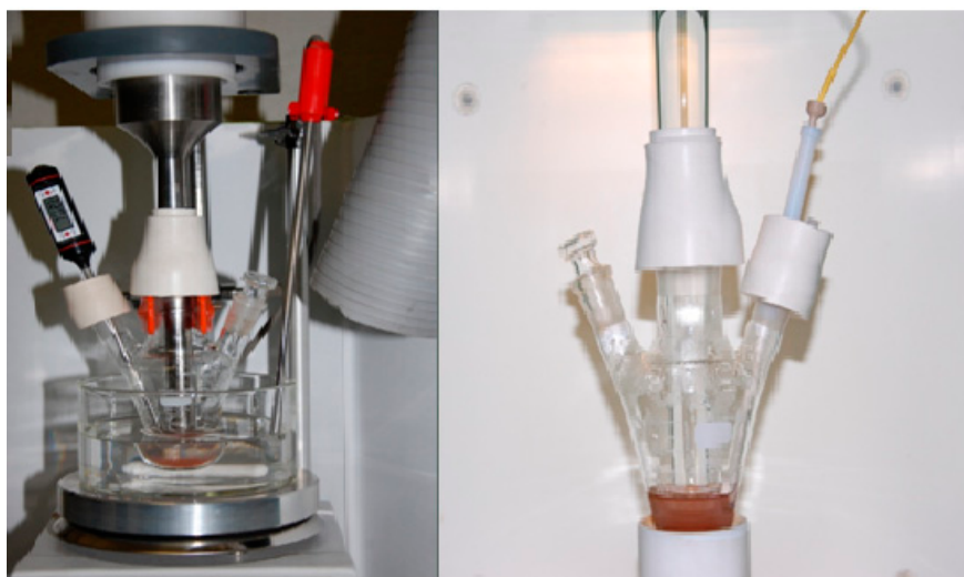
Figure 1. Click cycloadditions with metallic copper activated by ultrasound alone ( left ) and the combined action of US and MW irradiations in a professional MW reactor ( right ). Set-ups from Cravotto's group laboratory at the University of Turin.
