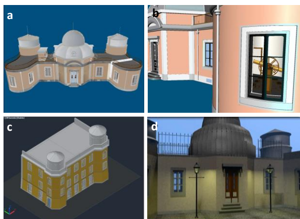
Figure 1: Astronomical Observatory of the Lisbon Polytechnic School: a) 3D model obtained from a TLS point cloud; b) A view into the meridian room with the meridian circle; c) Mathematics Building; d) 3D model obtained from scratch.
