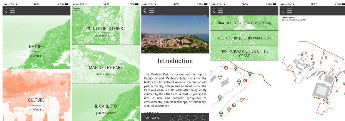
Figure 5. Screenshots of the app running. From left to right: the home page of the app, the menu from which the user can choose from among different categories, the textual information about a sample POI, the POIs alerted once the user gets within the beacon range, and the map visualization.
