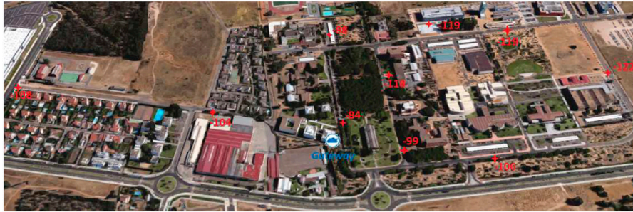
FIGURE 14 | Campus of the University of Extremadura in Badajoz, Spain, with the RSSI measured at different locations. Background image taken from Google Maps (2021).
