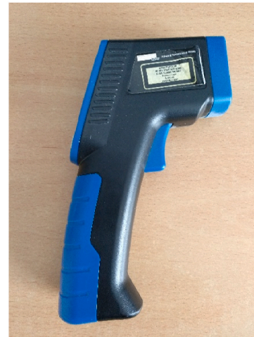
Fig. 1. Commercial infrared thermometer used in the present study.
