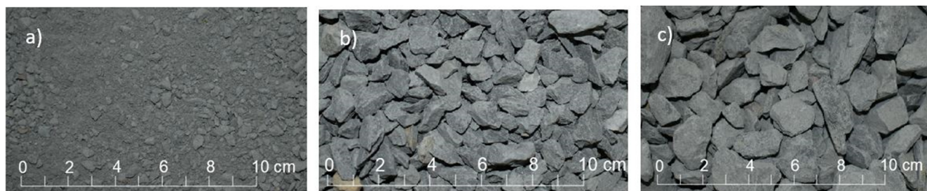
Fig. 1. a) Finely crushed stone (CS-F); b) medially crushed stone (CS-M); c) coarsely crushed stone (CS-C).
