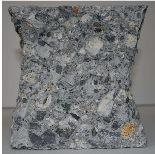
Figure 10. Failure mode in HR-100+50 mix.
