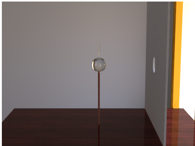
Fig. 3. Simulation of a flask filled with water in front of a white screen with an aperture (sunlight coming from the right).
