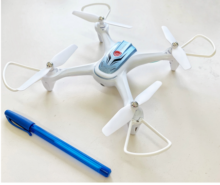
Figure 5: Drone used in the experimental tests. Syma X15W - wingspan: 31 cm, size: 22 \times 22 \times 5 cm 3 .
