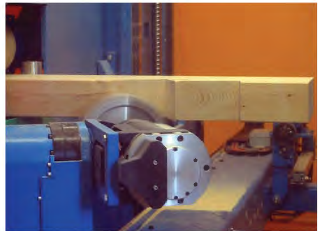
FIGURE 2. Computer-aided manufacturing (CAM) of notches for a double-step joint.
