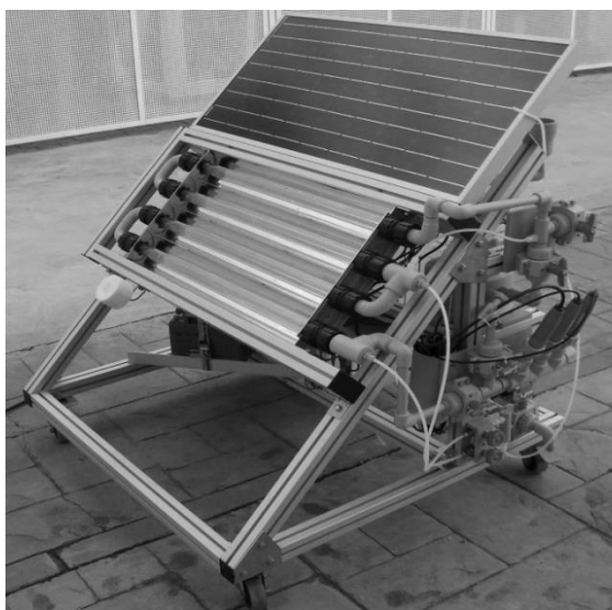
Figure 2.5. CPC photo-reactor used in pilot scale experiments
