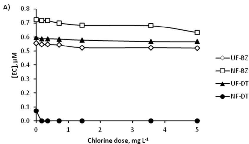
Figure 1. Concentration profiles of BZ and DT during a) chlorination of permeates obtained after the filtration pre-treatment (UF or NF) of SW water.
