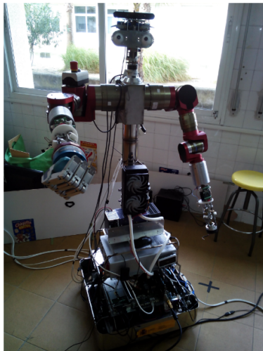
Figure 1.2: Humanoid robot Loki in Robolab, which was used in the attempt to calibrate the solution to the Inverse Kinematics problem by using GTSAM.
