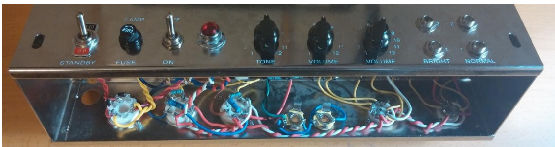
Ilustración 65. Interconnection of all circuit elements. Twisted wiring.
