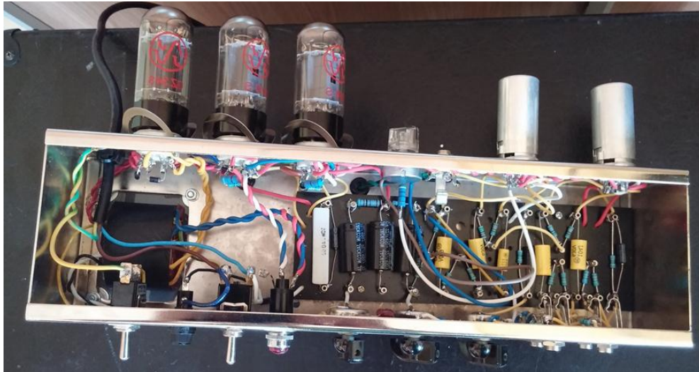
Ilustración 71. Global view with valves mounted on the chassis.
