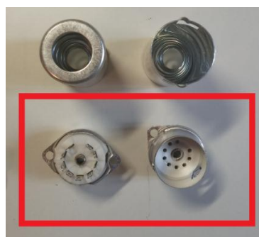
Ilustración 69. Protector valve (above) and ceramic sockets (below) used in the installation of valves pre-amplification in the chassis.
