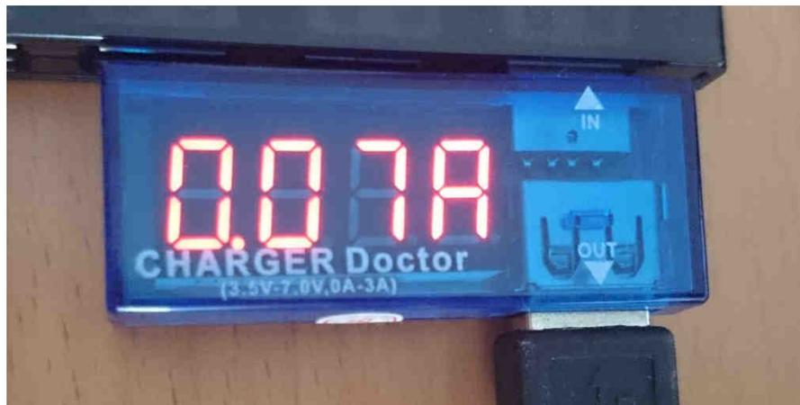
**Figure 31 Working system current consumption**
