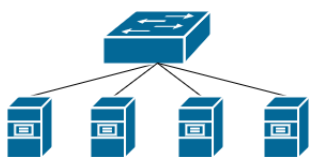
Figure 3.11: DCell-0 with 4-port switch.
