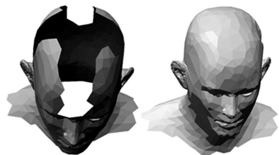
Fig. 2. Example of hole-filling by unfolding the mesh. The method presented by Brunton et al. (2009).
