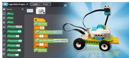
Figure 3.1: Lego WeDo 2.0 robot and code example
