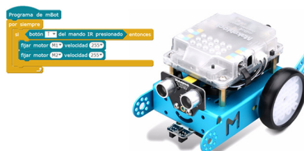
Figure 3.3: Mbot robot and programming example
