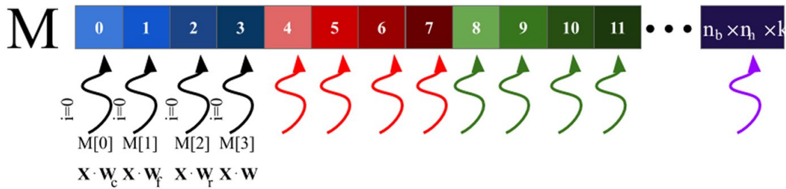
Fig. 3 Diagram illustrating the threads' access to auxiliary matrix \mathbf{M} , where black, red green and purple arrows represent those threads with identifier 0, 1, 2 and n_b \cdot n_h - 1 , respectively
