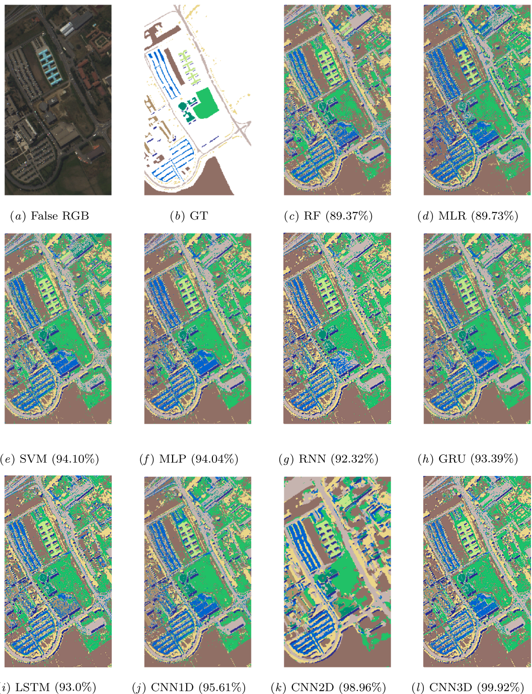
Fig. 13. Classification maps for the UP dataset with 10% of training data. Images from (a) to (j) provide the classification maps corresponding to Table 7. The corresponding overall classification accuracies (OAs) are shown in brackets.
