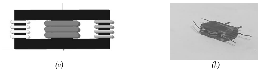
Figure 56. FEM and tested Model. Component III (a) FEM model; (b) Tested Model.
