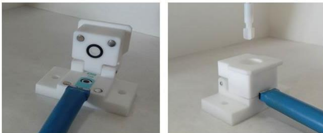
Figure S2. Voltammetric teflon conic cell, specially designed to perform analysis on screen-printed platforms (up to 2 mL solution volume).
