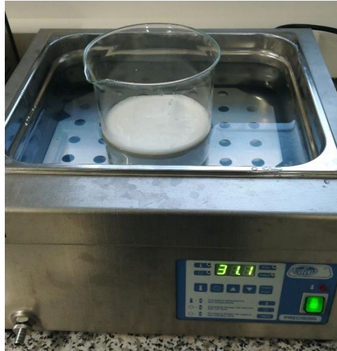
Figure 3. Thermostatic bath JP SELECTA mod. PRECISDIG used during the coagulation phase of milk (31 °C, 20 min).
