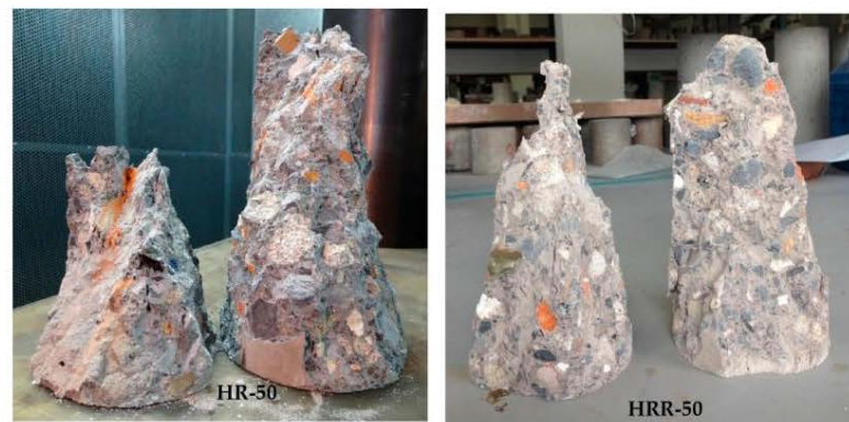
Figure 12. Fracture surface of samples broken during fatigue tests.
