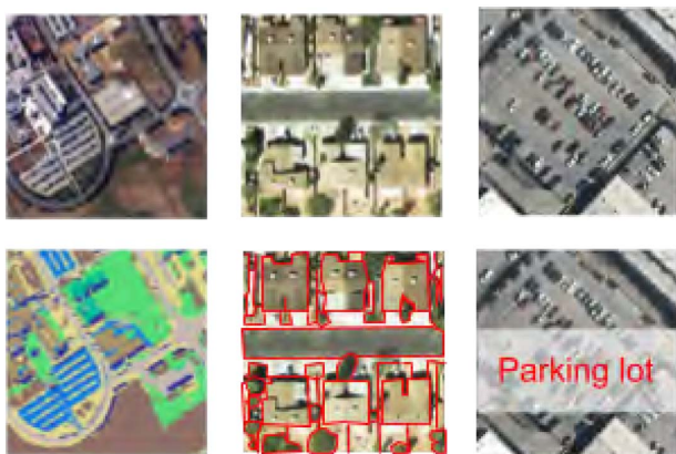
Fig. 1. Remote sensing classification can be tackled at three different levels: pixel-level (left), object-level (center), and scene-level (right).
