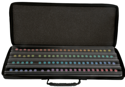
FIGURE 5. Original Farnsworth-Munsell 100 Hue test samples divided into four rows.
