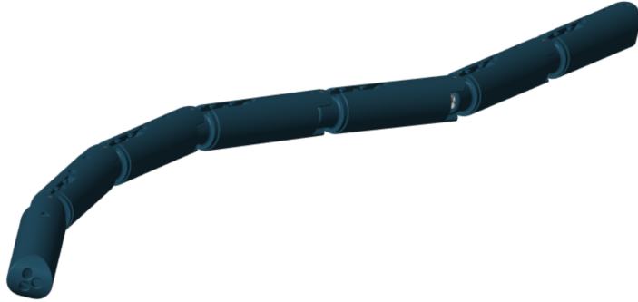
Figure 5.2: 6-link eukaryotic flagellum swimming robot.
