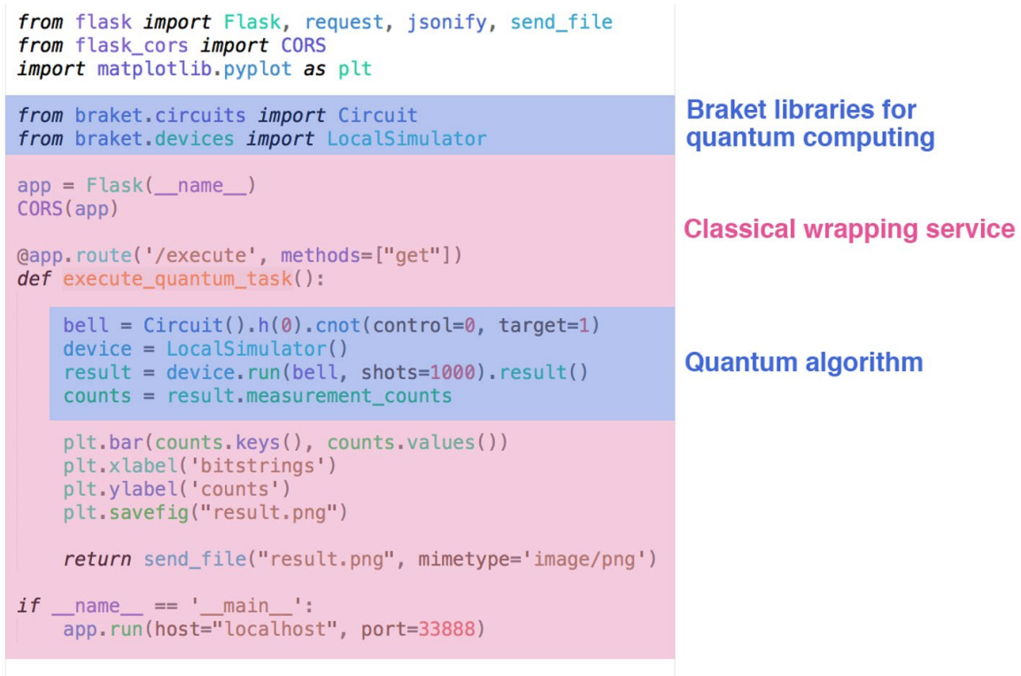
Fig. 2 Quantum algorithm wrapped by a classical service
