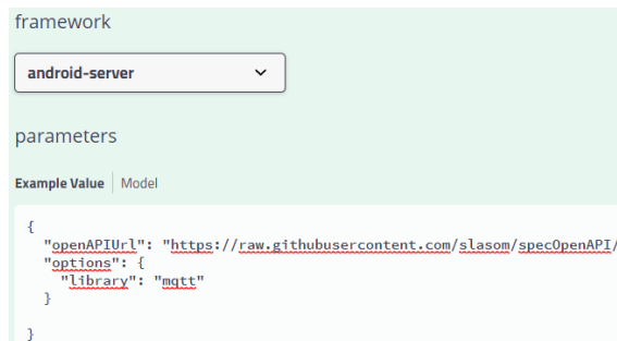
Fig. 2. Parameters to generate the Android application using the MQTT library.
