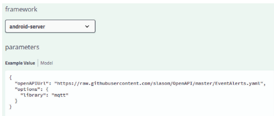
FIGURE A3 Parameters to generate an application using MQTT
