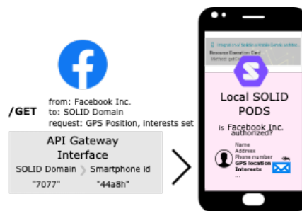
Fig. 2. Process to obtain GPS value and interests data from user PODS.
