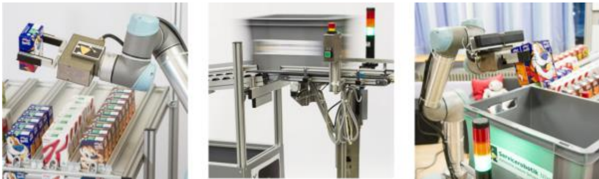
Figure 33. Intralogistics Industry 4.0 Robot Fleet Pilot. (Left) Picking items. (Middle) Transport and autonomous delivery of boxes with goods. (Right) Order picking into boxes. (Source: https://robmosys.eu )
