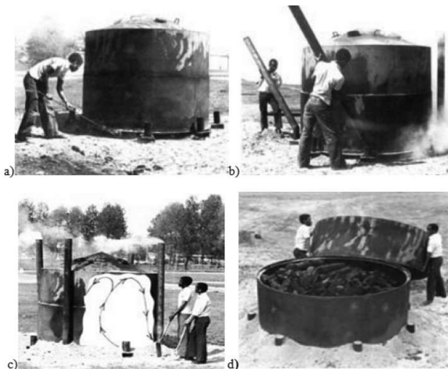
Fig. 1. Photograph of a typical artisanal charcoal kiln for holm oak prunings taken in Zahinos (Badajoz, Extremadura, Spain); a) Kiln ignition; b) Location of chimneys for fumes; c) Circulation of gases; d) Obtaining charcoal from holm oak prunings. Adapted from Tropical Products Institute (TPI), www.fao.org .
