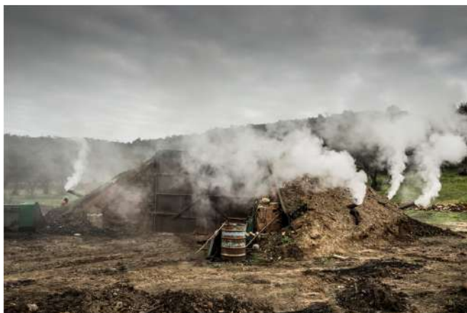
Fig. 1. Photograph of a typical artisanal earth-mound oak-wood charcoal oven taken in Zahinos (Badajoz, Extremadura, Spain).
