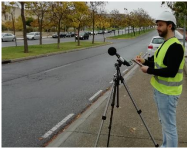
(a) Step 1 – Perform measurement with app or soundmeter
