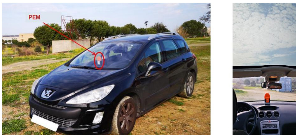
Fig. 2. Left: Exterior view of the vehicle with the exposure meter. Right: View of the position of the PEM from inside the vehicle with the panoramic roof open.
