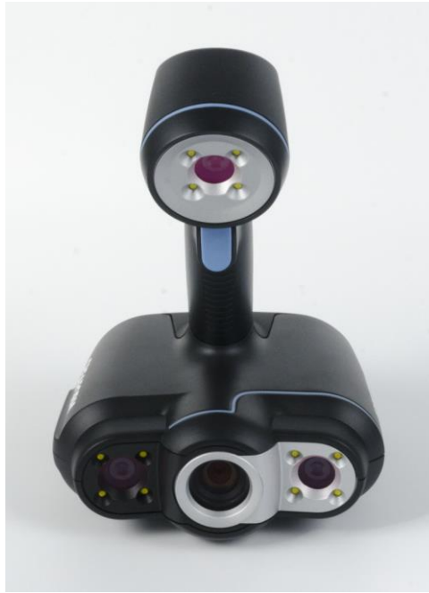
Figure 1. The Go!SCAN scanner has three cameras; two cameras (upper and lower right) capture the deformation of the pattern and generate a point cloud, with possibility of texture information using the third camera (left). The light-structured emitter is between the two bottom cameras.
