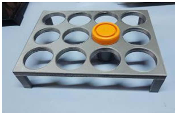
1 2 3 4 5 6 7 8 9 10 11 12 104 13 14 105 Figure 1. Adapter designed in 3D to be incorporated into a thermostatic bath.
