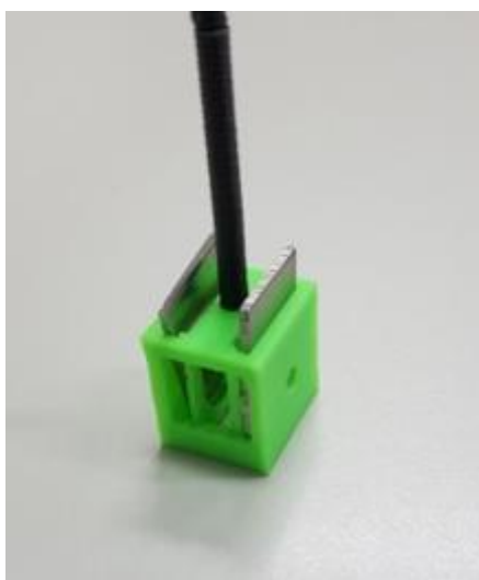
Figure 2. System of integrated electrodes (designed in 3D).
