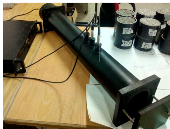
Figure 6. Impedance tube with 100 mm internal diameter.
