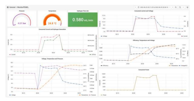
Fig. 6. General view of the Grafana interface for PEMEL monitoring.
